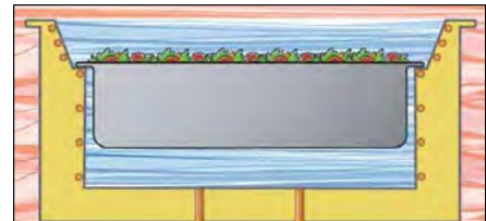
From inside the cavity, the beveled edge allows cold air to effectively blanket your food product
