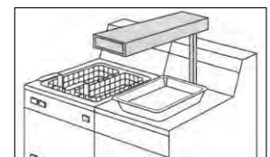
GRFS, GRFSL, GRFSC, GRFSL with swing-away post mount and cord with plug
